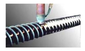
The regeneration of screws is performed using the extremely wear-resistant welding filler materials that we have developed ourselves on a 7 axis controlled CNC PTA welding plant.
